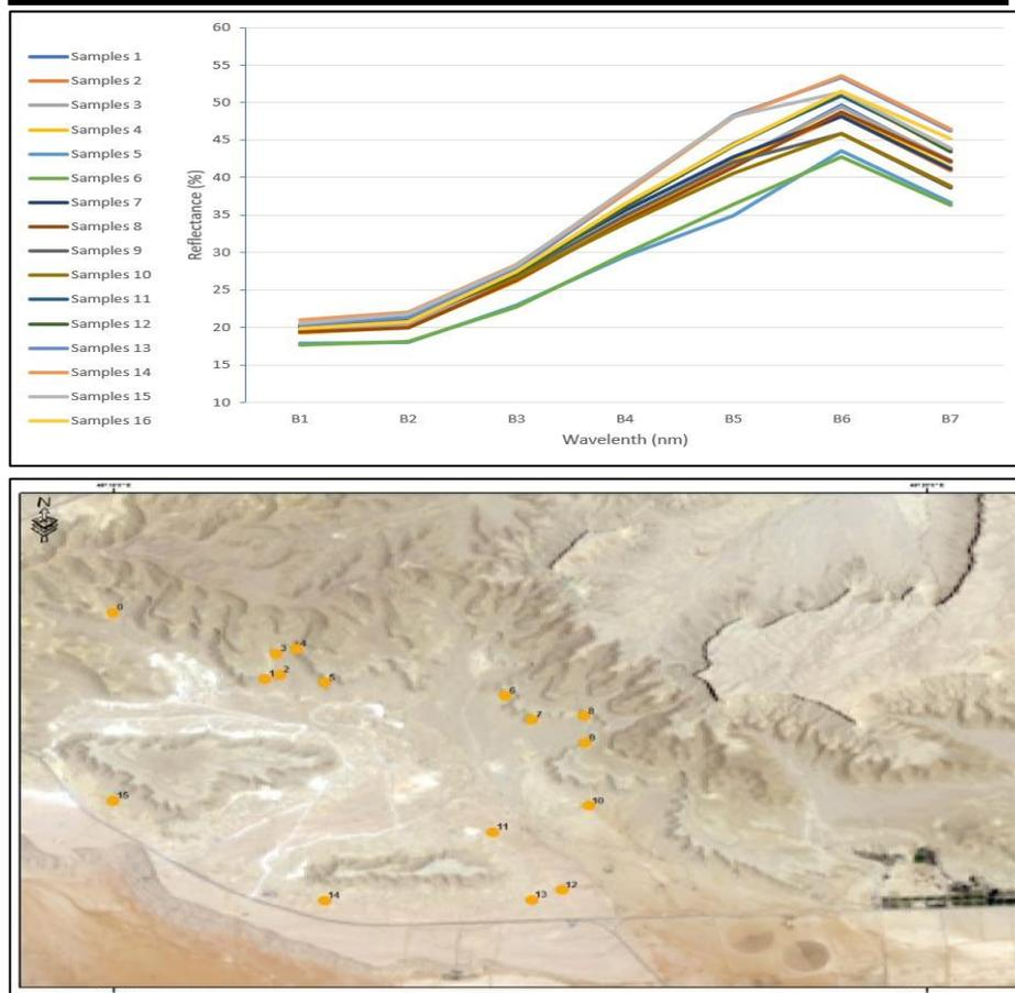
**Figure 11. Spectral values of the Limestone rocks samples, produced by ArcGIS**
